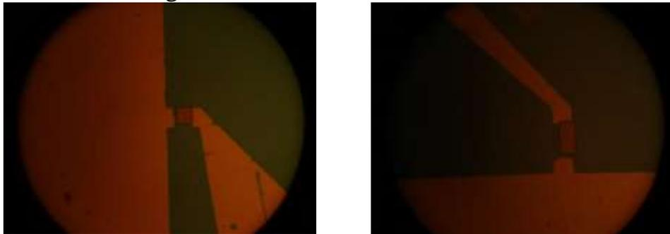
Figure 5. Graphene patterning mask, (Rectangular 60×56 μm<sup>2</sup> & 30×56 μm<sup>2</sup> with photoresist), to protect graphene in O<sub>2</sub> plasma process.
