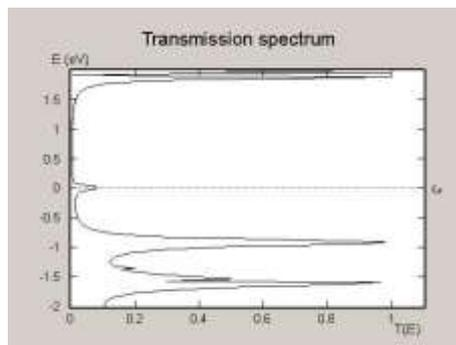
Figure 8. Transmission spectrum of the GRFET with a gate potential of -1 Volt.
