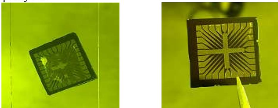
Figure 3. Transfer graphene/PMMA stack on Si/SiO<sub>2</sub>/Cr markers substrate with water bubbles. Backe the Si/SiO<sub>2</sub>/Cr markers/graphene/PMMA for evaporate water bubbles and improve the contact between the stack and the substrate.
