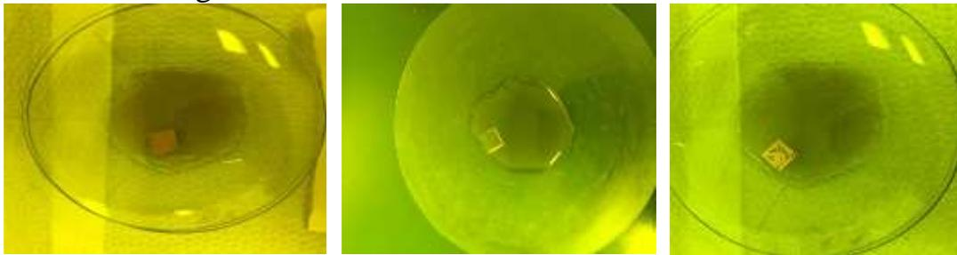
Figure 2. The etching of copper foil, PMMA/graphene stack floats on the solution surface.
