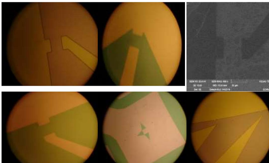
Figure 1. Alignment Maskers Mask, the SEM image and optical microscopy images of the aligning markers electrodes. (Si/SiO<sub>2</sub>/Cr Markers).
