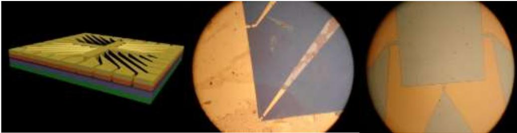
Figure 7. A) The mask of the source and drain electrodes, (31 transistor samples with different dimensions). B) Optical microscopy images of the source/drain contacts.
