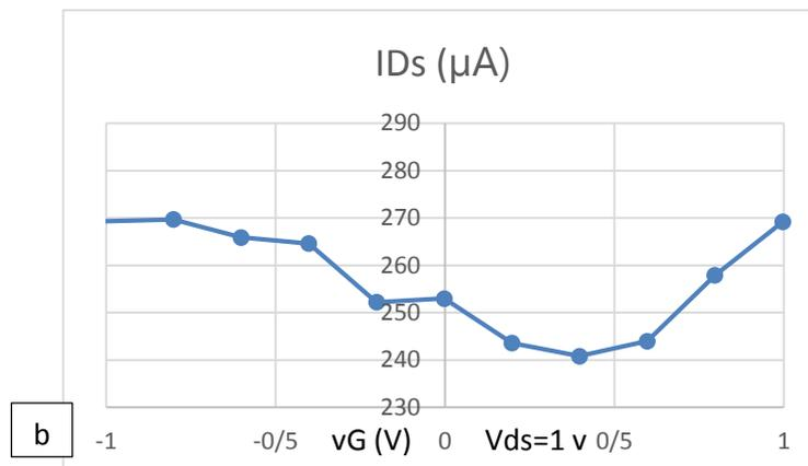
Figure 9. Electrical properties of a GFET. a) Id-Vd curves measured at various Vg with Vd sweeping ranges. b) Typical V-shape bipolar property output.
